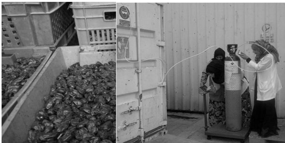
Fig.10- Setup of container fumigation of dates with ECO 2 FUME ® in the Sultanate of Oman.
