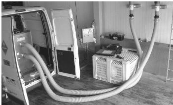
Fig. 8- The HDS 800 in a fumigation van with a two-hose connection to a fruit fumigation chamber.
