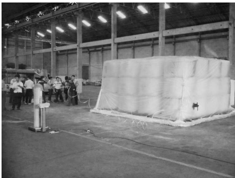
Fig. 6- Setup of tarpaulin fumigation of rice in jumbo bags in one of the rice mills in Thailand.
